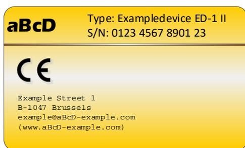
Template of a correct data plate from manufacturer using a (registered trade) name:
